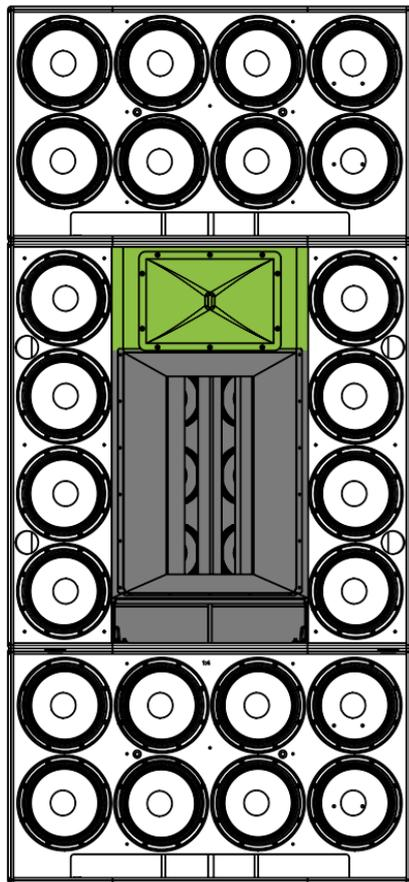
To cover very large crowds you need a large system capable of delivering high SPL, running multiple components. To do this, as one large point source enclosure is somewhat difficult as it would be almost impossible to move around or transport.
